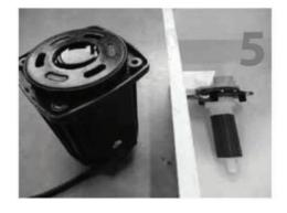
Put pumphouse in a vertical position and fill with a mild lime scale remover (like cleaning vinegar). Immerse rotor in a plastic bowl/container filled with the same lime scale product and leave both for 24 hours. After 24 hours rinse off with water and re-assemble pump.
