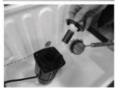
Remove rotor from pump house and clean with water and brush
